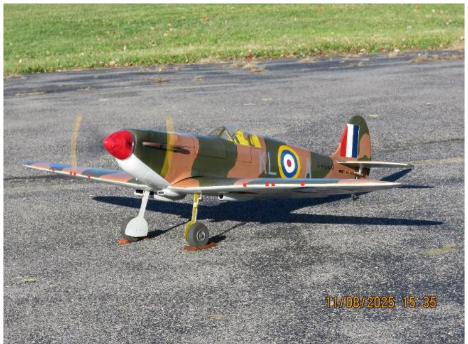
Gary Brown built his Spitfire Mk 1 from enlarged Model Builder plans. The RC conversion is electric powered with retractable landing gear from E-flite.
